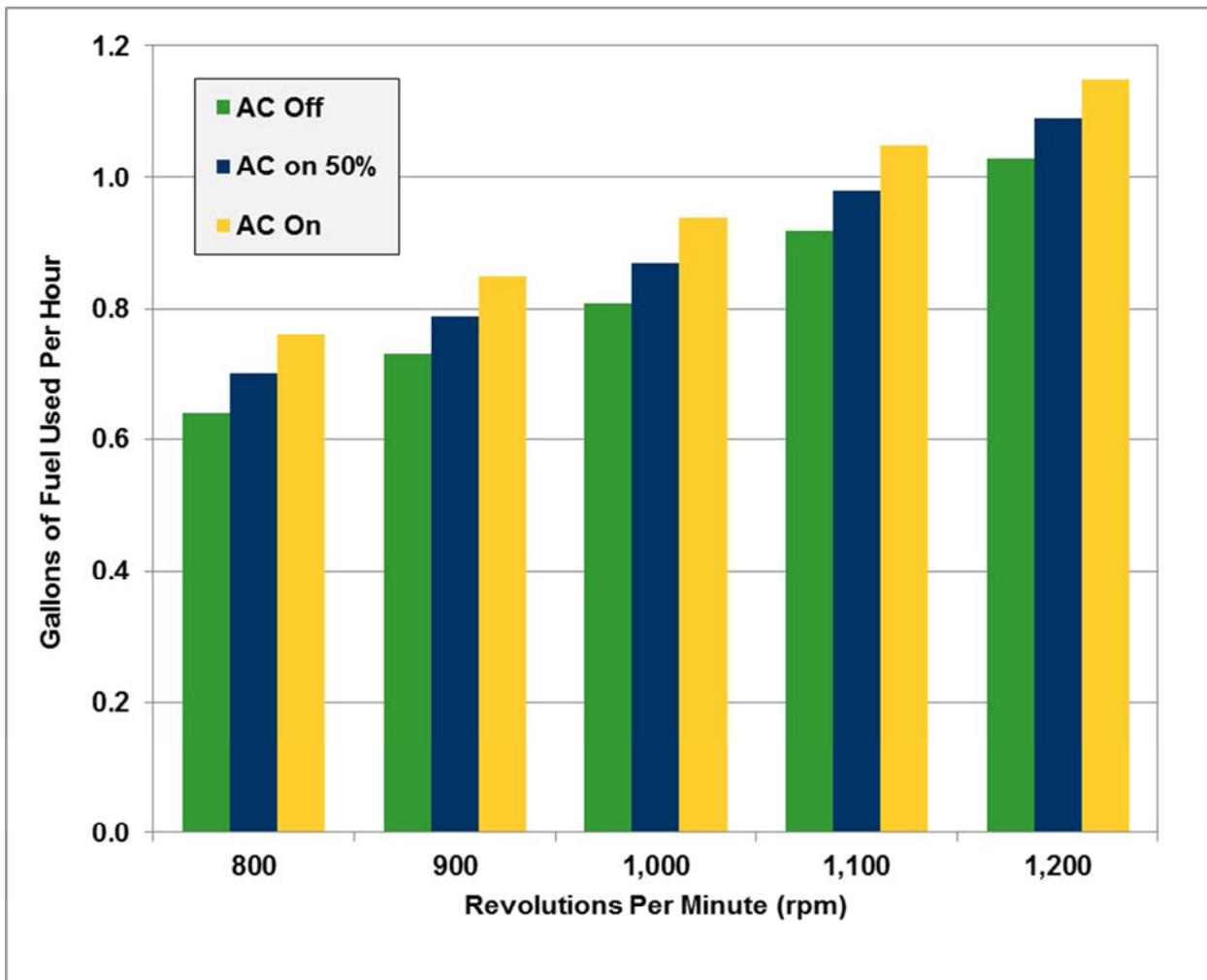
FIGURE 68. Average Amount of Fuel Used for Idling a Truck-Tractor
