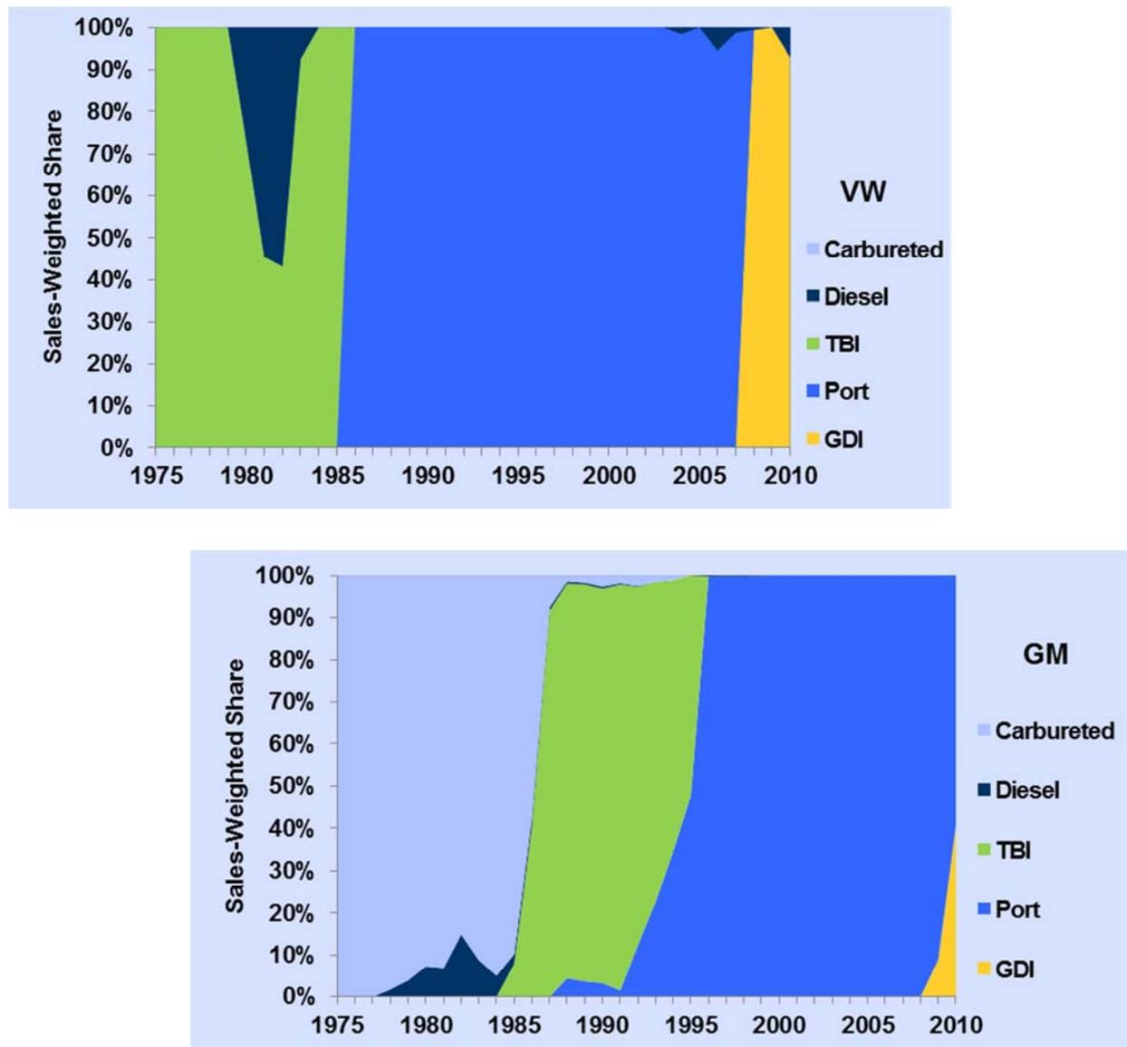
FIGURE 48. Light Truck Fuel Metering for Selected Manufacturers, 1975-2010
