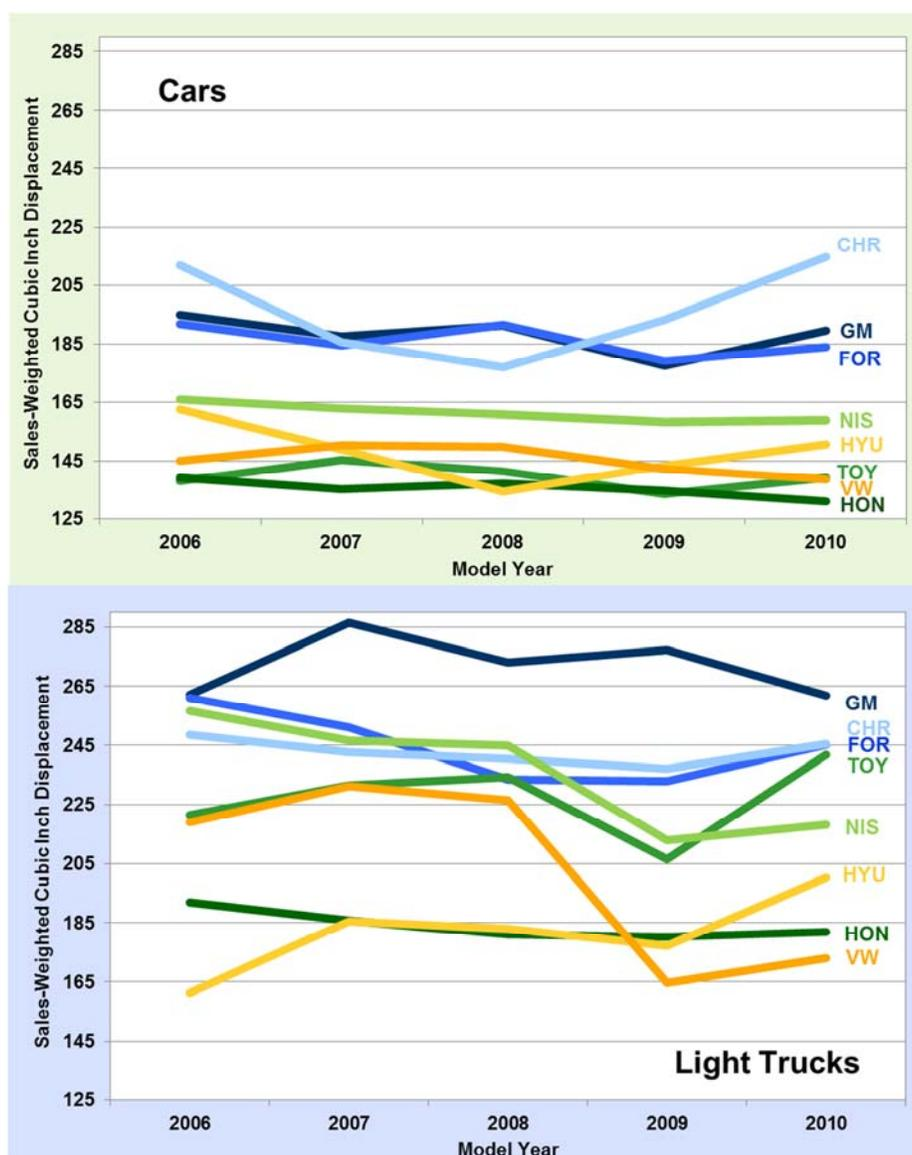
FIGURE 39. Car and Light Truck Engine Size by Manufacturer
