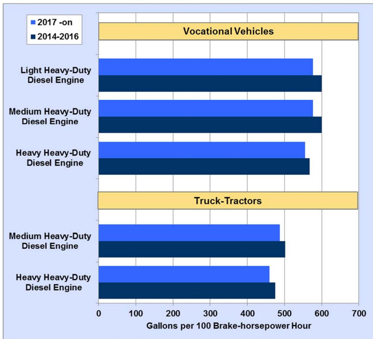
FIGURE 100. Fuel Standards for New Diesel Engines
