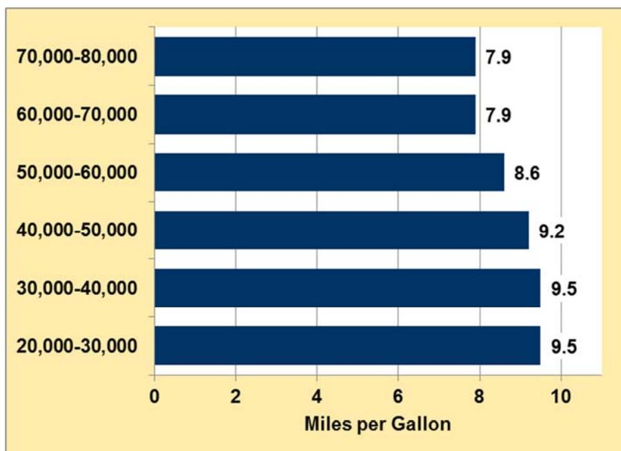
**FIGURE 66. Fuel Efficiency of Class 8 Trucks by Vehicle Weight Range on Flat Terrain**
