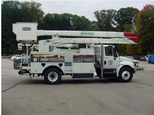
**FIGURE 81. Hybrid Bucket Truck**
