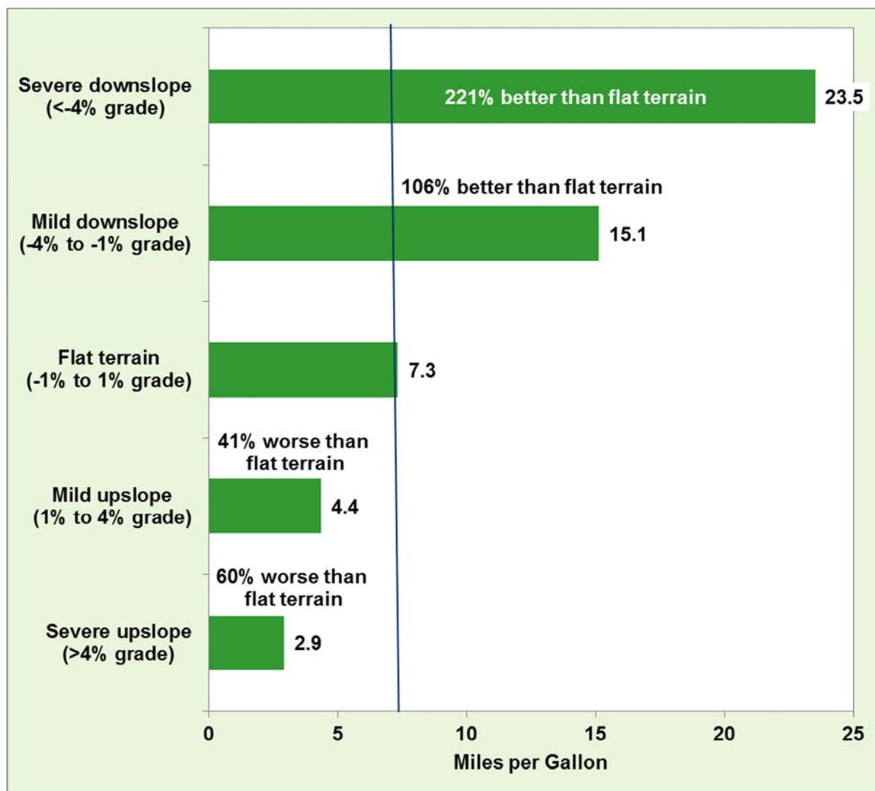
FIGURE 67. Fuel Efficiency of Class 8 Trucks by Roadway Grade
