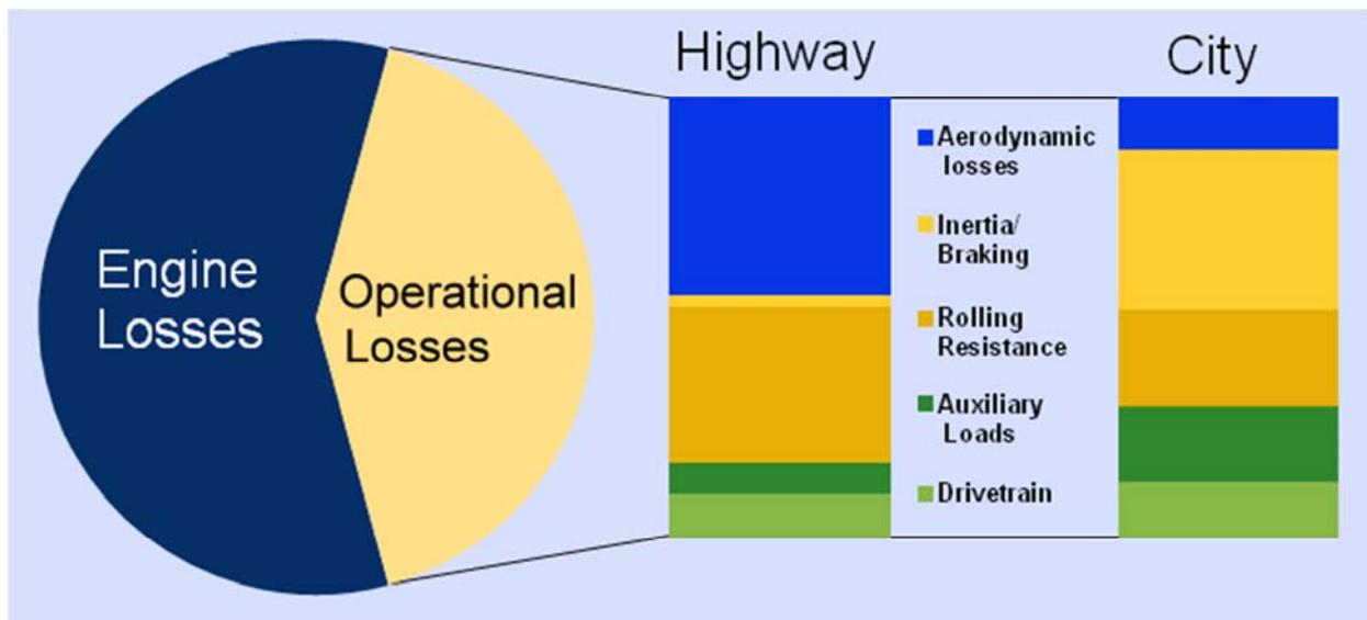
FIGURE 84. Class 8 Truck-Tractor Energy Losses
