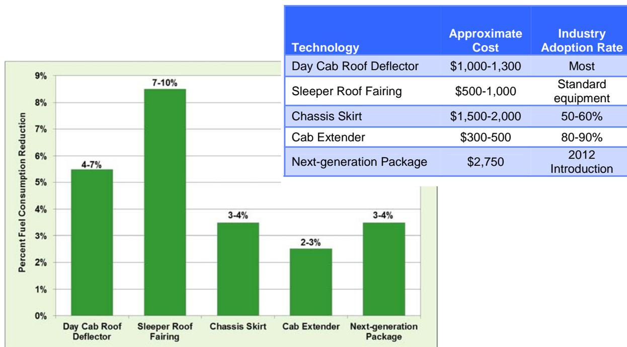
**FIGURE 85. Fuel Consumption Reduction Rate, Approximate Cost, and Industry Adoption Rate for Aerodynamic Technologies**
